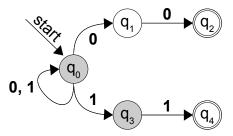
Finally, we process the last character, a **1**. State  $q_0$  transitions to  $q_0$  and  $q_1$ , and state  $q_1$  transitions to state  $q_4$ . We thus end up in this final configuration:
