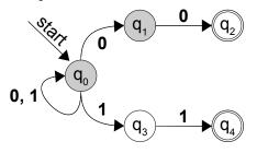
Next, we process the second character (**0**). From state  $q_0$ , we transition into  $q_0$  and  $q_1$ , and from state  $q_1$  we transition into  $q_2$ . We thus end up in states  $q_0$ ,  $q_1$ , and  $q_2$ , as shown here:
