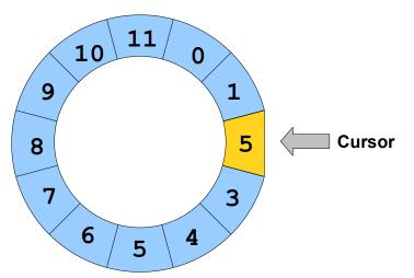
There is a particularly elegant construction which enables us to build a ring buffer out of a deque. The basic idea is to "unroll" the ring buffer into a linear sequence, then use a combination of push\_front, pop\_front, push\_back, and pop\_back to simulate moving the cursor to the left or to the right. This technique of simulating one data structure using another is ubiquitous in computer science, and many important results in computability theory use constructions of this form.
