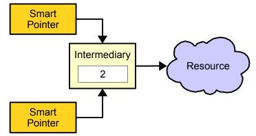
Although in this diagram we only have two objects pointing to the intermediary, the reference-counting system allows for any number of smart pointers to share a single resource.
