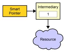
Finally, suppose this last smart pointer needs to stop pointing to this resource. It decrements the reference count, but this time notices that the reference count is zero. This means that no other smart pointers reference this resource, and the smart pointer knows that it needs to deallocate the resource and the intermediary object, as shown here:
