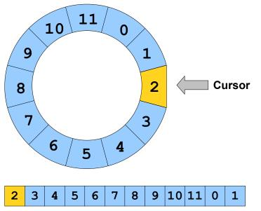
Similarly, to move the cursor one step counterclockwise, we move the element at the end of the deque onto the front, as shown here:
