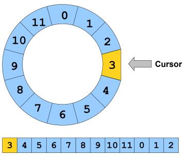
Write a pair of functions CursorClockwise and CursorCounterClockwise which take in a deque representing a ring buffer and update the deque by simulating a cursor move in either direction. Then write functions CursorRead and CursorWrite which read and write the element stored at the cursor. You've just shown how to represent one data structure using another!
