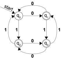
As with the previous DFA, this DFA has four states, but notice that three of them are marked as accepting. This leads into the second important detail regarding DFAs – the DFA only accepts its input if the DFA ends in an accepting state *when it runs out of input*. Simply transitioning into an accepting state does not cause the DFA to accept. For example, consider the effect of running this DFA on the input **0101**. We begin in the start state, as shown here:
