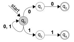
We now process the first character of input (0) and find that there are two transitions to follow – the first to  $q_0$  and the second to  $q_1$ . The NFA thus ends up in both of these states simultaneously, as shown here:
