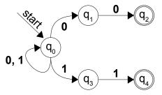
Here, the start state is  $q_0$  and accepting states are  $q_2$  and  $q_4$ . Notice that the start state  $q_0$  has two transitions on **0** – one to  $q_1$  and one to itself – and two transitions on **1**. Also, note that  $q_3$  has no defined transitions on **0**, and states  $q_2$  and  $q_4$  have no transitions at all.
