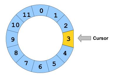
A ring buffer consists of a circular ring of elements with a *cursor* which selects some particular element out of the buffer. The four main operations on a ring buffer are as follows:
