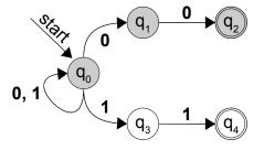
We now process the third character of input, which is a 1. From state  $q_0$  we transition to states  $q_0$  and  $q_3$ . We are also currently in states  $q_1$  and  $q_2$ , but neither of these states has a transition on a 1. When this happens, we simply drop the states from the set of current states. Consequently, we end up in states  $q_0$  and  $q_3$ , leaving us in the following configuration:
