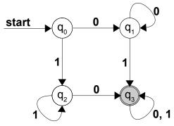
The final character of input is also a 1, so we follow the transition labeled 1 and end back up in q<sub>3</sub>:
