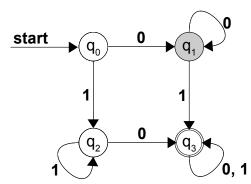
The second character of input is also a  $\mathbf{0}$ , so we follow the transition labeled with a  $\mathbf{0}$  and end up back in state  $q_1$ , leaving us in this state:
